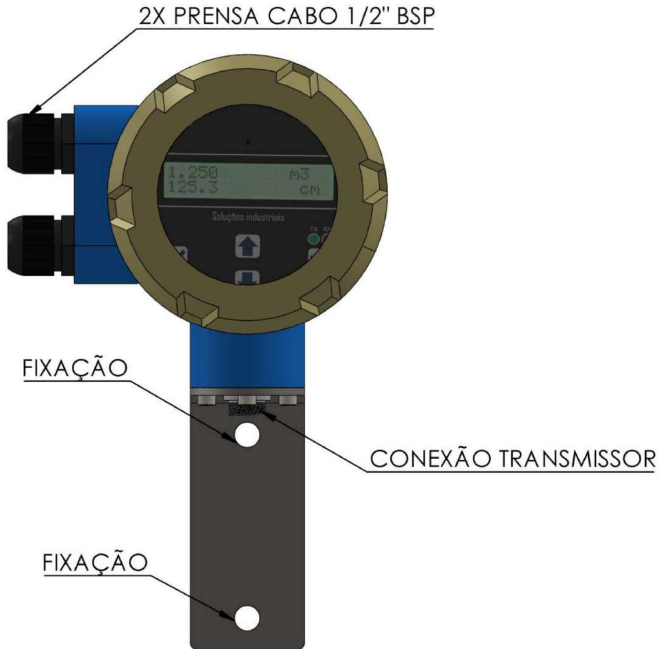
*Figura 1: MGG-Radar-R-T-R Conversor vista frontal*
